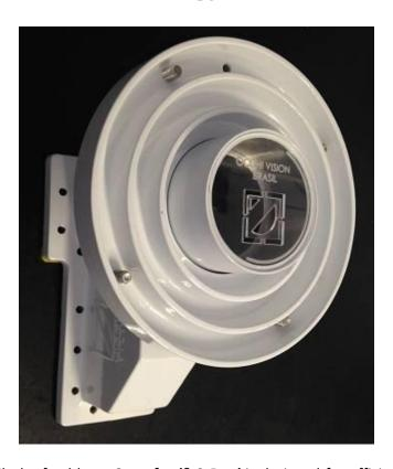
Produced in Brazil, the feed horn *Superfeed® 3 Dual* is designed for efficient and practical C Band reception, for use in professional satellite reception systems. The difference of this model is that both ports are in the same axial alignment, with Port 1 with direct reception and Port 2 with lateral reception.
